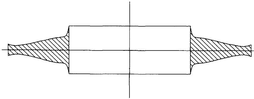
Fig. 7. Optimal shape mode  $m = 5$ ,  $a/b = 0.5$ , gain = 1.19.
